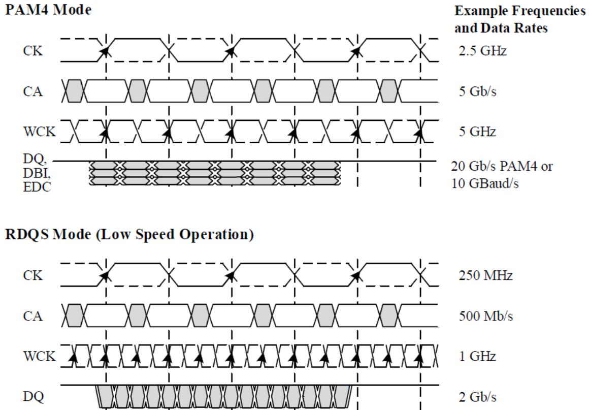
**Figure 6: Clocking and Interface Relationship**
